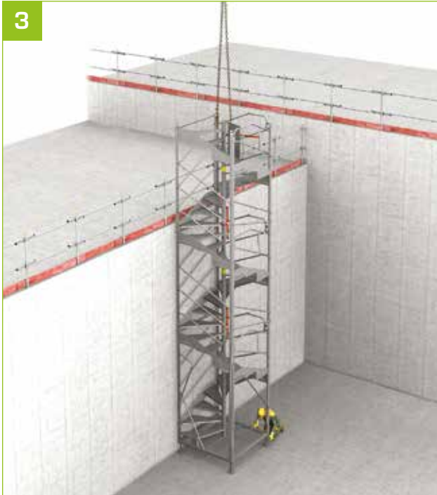
- Ground positioning and levelling of EscAlphi MDS.
