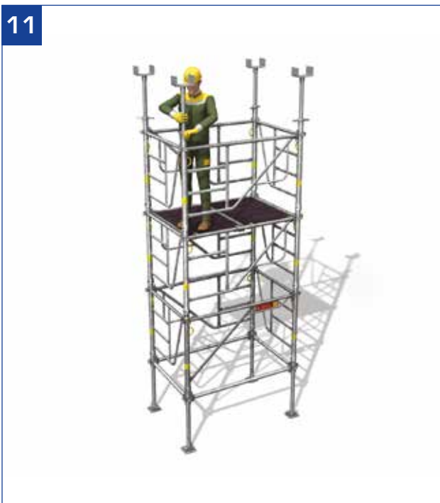
- Set up and adjust the head jacks.
