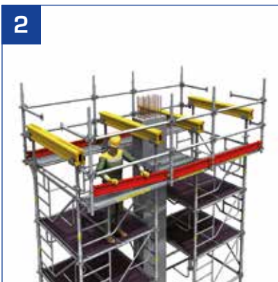
- Installation of brackets, risers, connectors, 0.30 m planks and baseboards.
