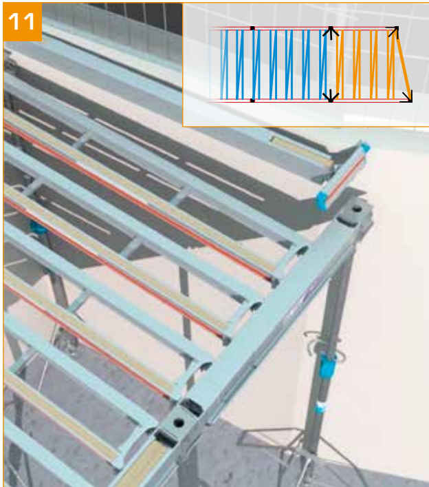
- Mount the secondary corner beam.
